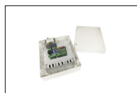
B71/PBX36/BOX/115 Hybrid inverter, "Network Assisted" version, for powering the automation. Also provides a battery-charger function thanks to the connection to the solar panels or mains supply for powering the 36V DC brushless digital controllers with a mains voltage of 115V AC.
