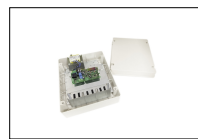
B71/PBX36/BOX Hybrid inverter, "Network Assisted" version, for powering the automation. Also provides a battery-charger function thanks to the connection to the solar panels or mains supply for powering the 36V DC brushless digital controllers with a mains voltage of 230V AC.
