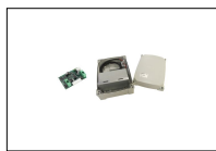
B71/BCHP/BOX Kit for emergency batteries charger for Brushless digital controller EDGE1/BOX - B70/1DCHP - B70/1THP 36V DC. Box case included and without recovery batteries.
